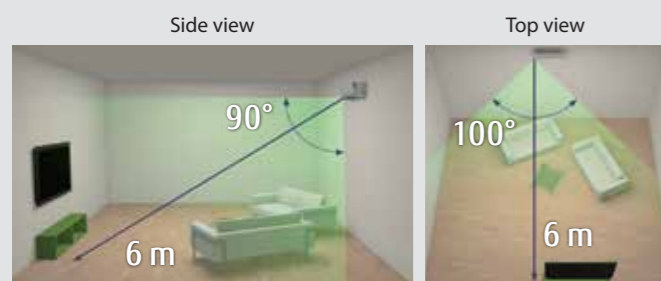
Detection range of Human Sensor
